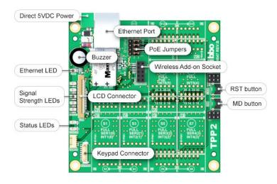
Each TPP can accommodate multiple Tibbit modules and connectors. Only bare essentials are provided on each boards: There is a CPU, an Ethernet port, and a very simple power supply. The rest of the board's functionality is defined by what Tibbits you
